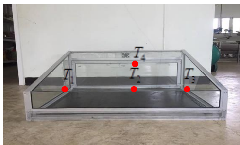
Figure 3 The position of type K thermocouple in solar dryer
